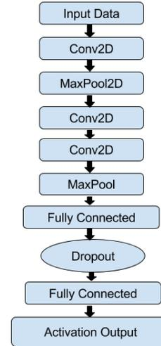
Fig. 7. The architecture of TFLearn Convolutional Neural Network
